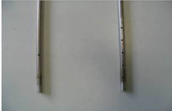
Figure 7 injection probe(L) and sampling probe(R) with multiple extraction points
