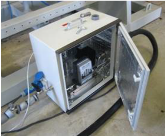
Figure 5 Coriflow in isolated (heated) cabinet with flexible hose
