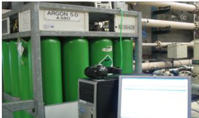
Figure 3 Ar-bottle stack used for the tracer tests
