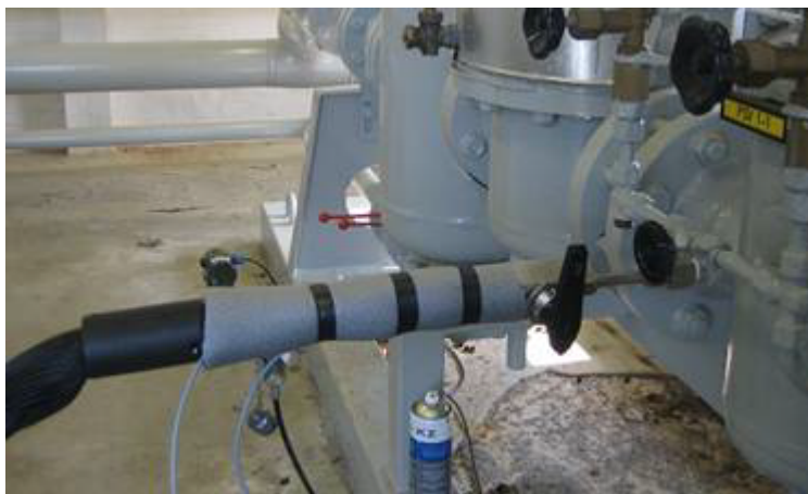
Figure 6 tracer-cord at sonic nozzle to inject the Argon with a constant temperature
